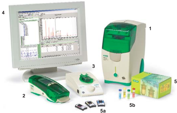
Fig. 1.1. The Experion system includes the following components: (1) Automated electrophoresis station, (2) Priming station, (3) Vortex station for RNA analysis, (4) System operation and data analysis tools, and (5) Analysis kits, which include the (a) chips and (b) reagents for protein (Pro260 kit), standard-sensitivity RNA (StdSens kit), and high-sensitivity RNA analysis (HighSens kit).
